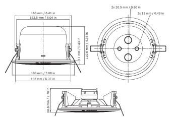
Mechanical diagram LC3-UC06 and LC3-CBB
